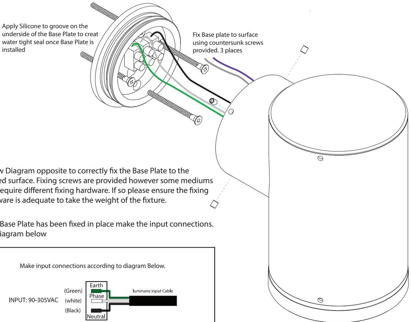
Follow Diagram opposite to correctly fix the Base Plate to the desired surface. Fixing screws are provided however some mediums may require different fixing hardware. If so please ensure the fixing hardware is adequate to take the weight of the fixture.
