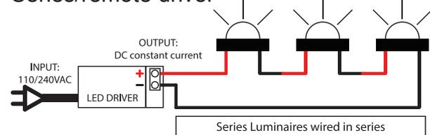
Diagrams are a guide only, wire colours and polarity may change depending on fixture and country
